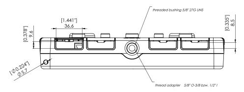
Rear view with mounting plate removed – cable duct:
